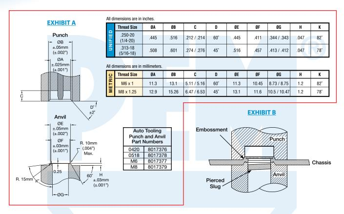
If not using in-die installation equipment, a fixture, template or some other location device should be used to be sure that the fastener is consistently located in the proper position on to the sheet.
