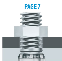
Flush, low-displacement head studs Types FHL/FHLS
